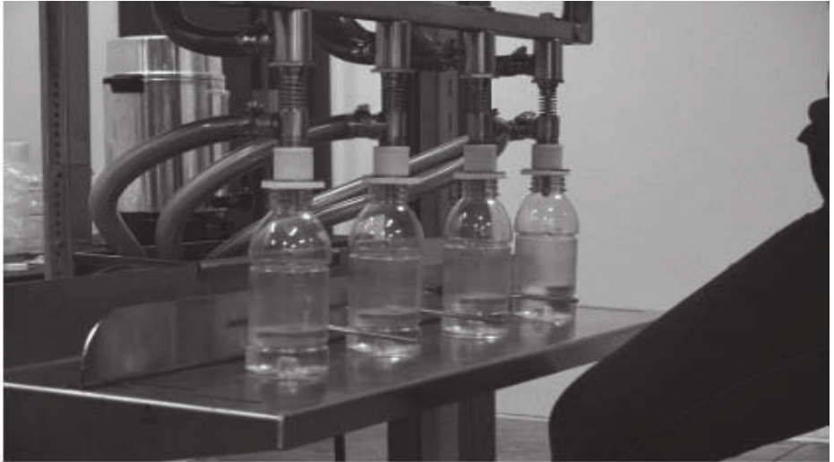
Figure 3. Acidified and thermally treated maple sap bottled using a water jacketed tank. This same unit is used for bottling maple syrup and similar bottling units are common in maple syrup production facilities. Photo by Ailis Clyne.
