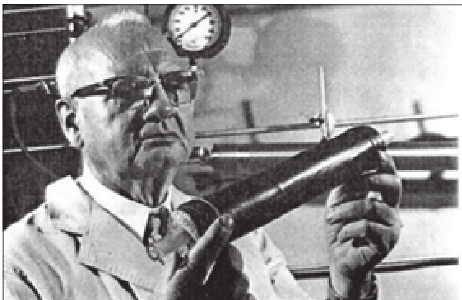
Figure 1 Dr. Willits of the USDA Eastern Regional Lab examining an experimental RO membrane (source: February 1969 Maple Syrup Digest).
