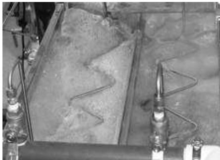
Figure 3. Effectiveness of the prototype to control foam formation in sap pans (left: prototype off; right: prototype on).
