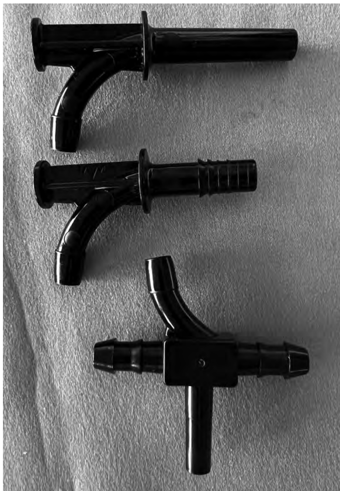
Figure 1. Spout and "tee" designs incorporating the arc-flow design. Standard 5/16" nylon spout (top) with Arc-Flow, Barb-spout with Arc-Flow (middle), and Arc-Flow Tee (bottom). For the Arc-Flow Tee, sap would flow from the lateral line from left to right. The dropline would connect to the curved segment of the tee at the top. The pin is located at the bottom (rather than coming out of the fitting towards the reader) to allow the fitting to be used on either side of the tree either in a normal configuration or in an inverted fashion (tapping below the lateral). University of Vermont Patents Pending.
