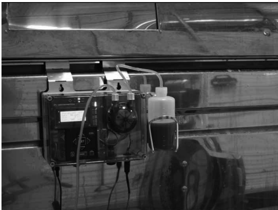
Automatic defoamer dispenser (probe not shown).
