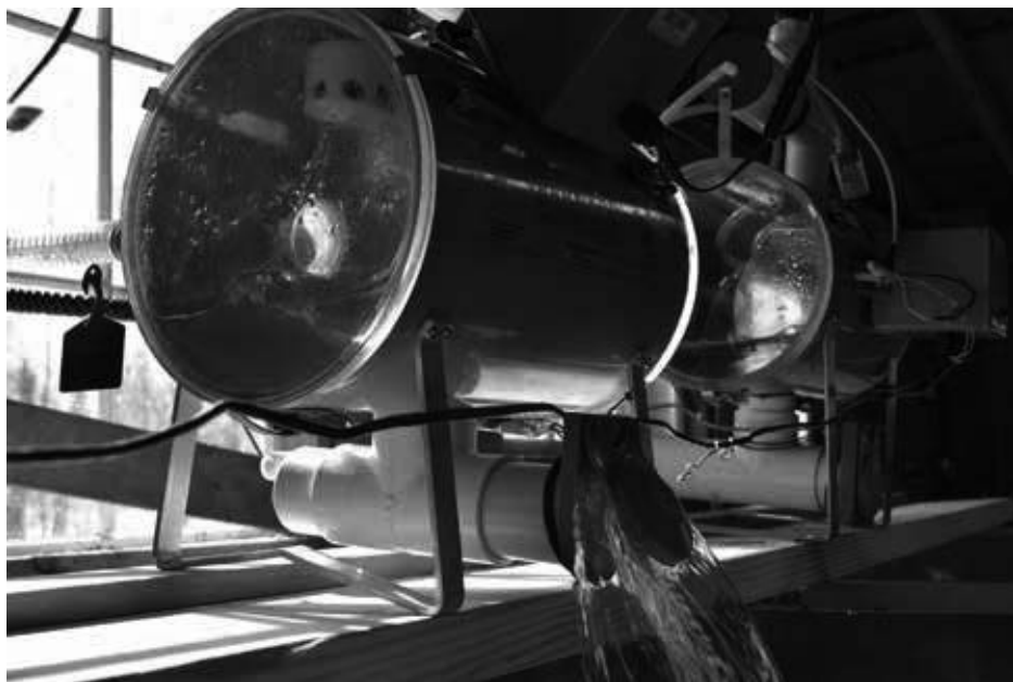
Figure 1. Two of the twelve mini-releasers used in this study. Each releaser was connected to 70-112 trees which made up a "treatment." Releasers were calibrated to a known volume of sap and are equipped with counters to allow calculation of the total amount of sap produced per tap each season for each treatment. Photo credit: Mark Is-selhardt, UVM Extension Maple Program.
