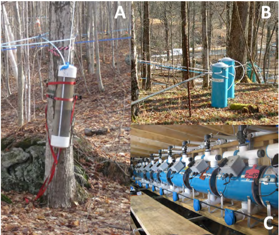
Figure 1. Various methods to measure sap yields from trees under vacuum conditions in sanitation studies. A) Single-tree vacuum chamber, B) Lateral line canisters for multiple trees (typically 3-5), and C) releasers connected to mainlines with 60-120 trees each.
