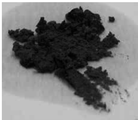
Figure 1: Sample of dried scale recovered from back pans of traditional evaporator.
