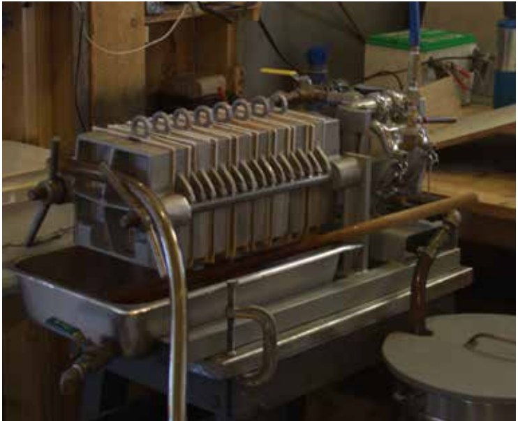
While gravity filtering is sufficient for small quantities of syrup, larger producers should use a filter press, which forces syrup through a series of plates lined with filter paper.
