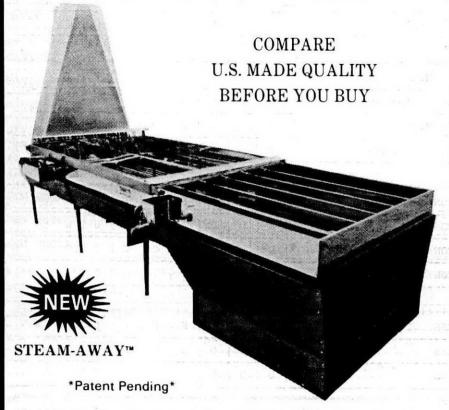
Our Steam-Away utilizes steam from the evaporator flue pan to increase evaporation. Test results show increased evaporation as high as 75%.
