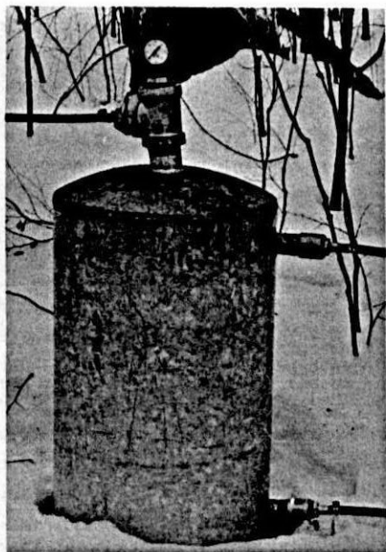
Figure 4. The vacuum-transfer tank is in the sugarcane. Sap flows from the trees on the left into the tank. The upper pipe on the right removes air from the tank, creating a vacuum, and sap travels out through the lower pipe.
