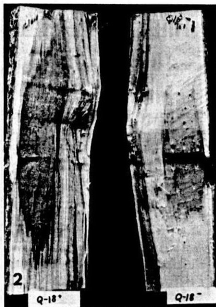
Figure 2. Dissection of two 20-month old tapholes, showing greater discoloration and decay in the pill-treated taphole (left) than in the control taphole (right).
