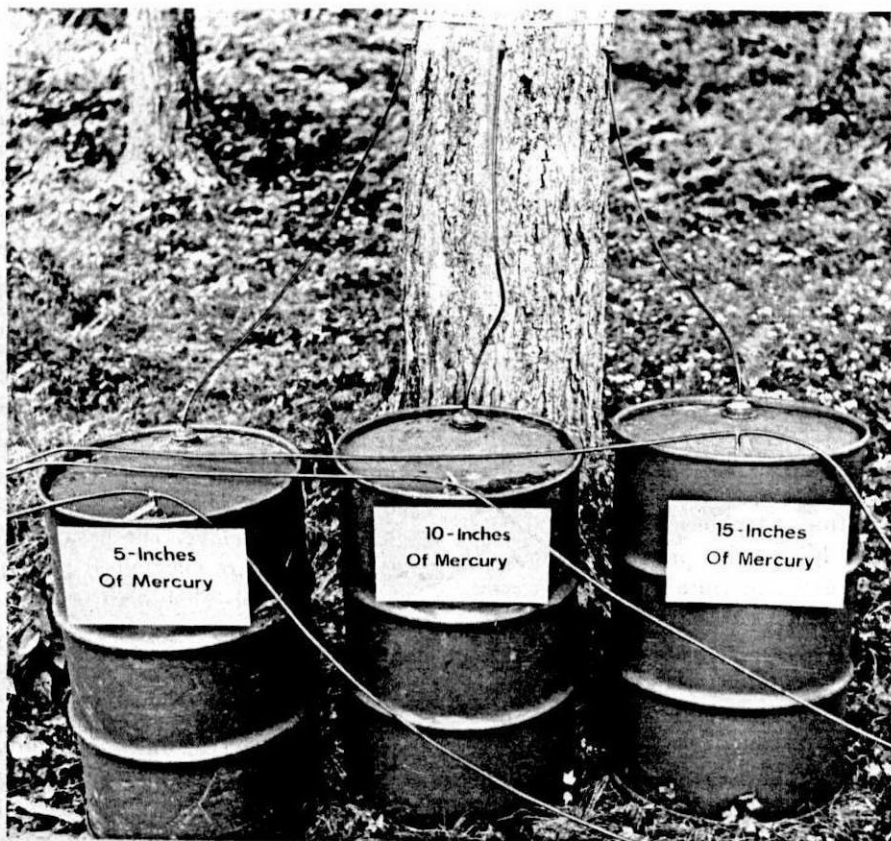
Figure 1. Sap from each taphole was collected in individually sealed 55-gallon steel drums.
