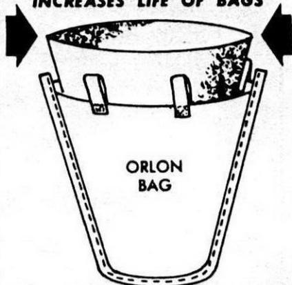
No need to remove filter bag from syrup filtering tank. Just remove liner from bag, rinse out solids in hot or cold water and replace. Liner has long life with careful use.
