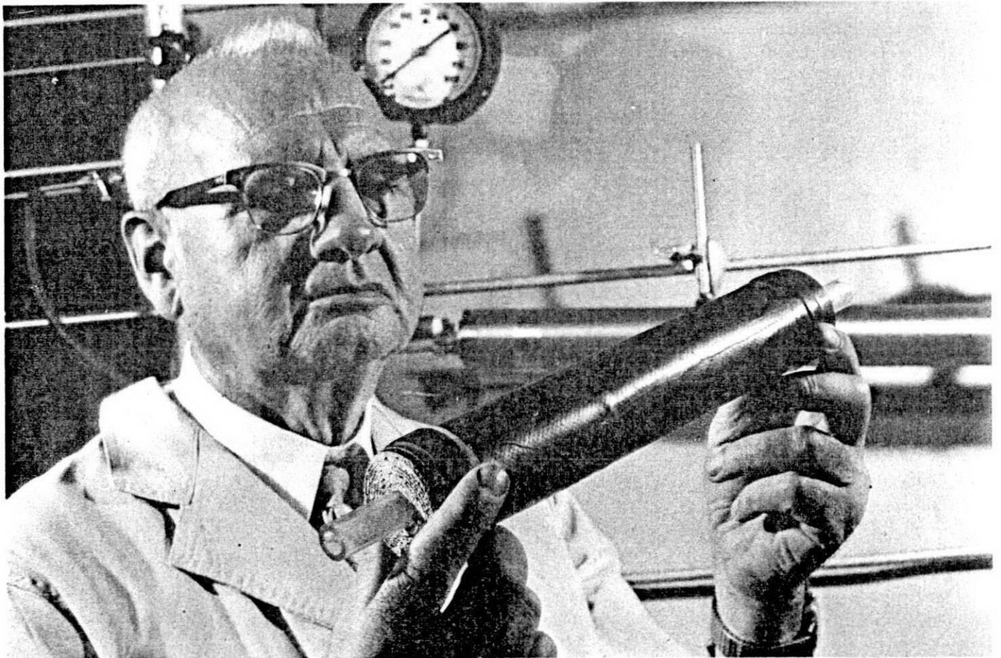
Dr. Charles O. Willits examining a module of a semipermeable membrane used to concentrate maple sap by reverse osmosis.
