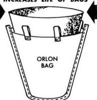
No need to remove filter bag from syrup filtering tank. Just remove liner from bag, rinse out solids in hot or cold water and replace. Liner has long life with careful use.
